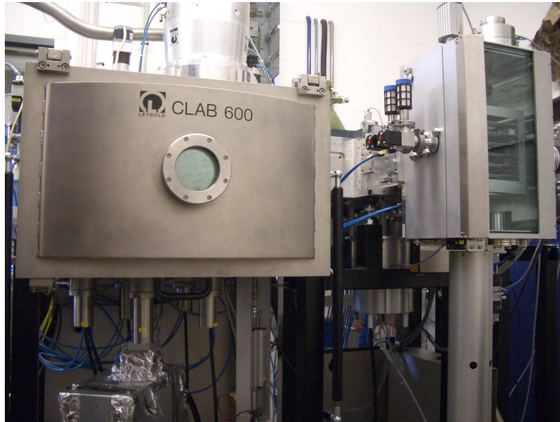
(a) Commercial sputter system CLAB 600, made by LEYBOLD
